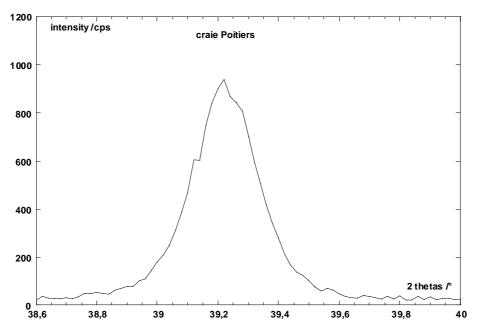
A careful examination of the PDF sheet and the experimental d-spacing show a systematic shift between these values. This shift can be assigned to a sample displacement.
